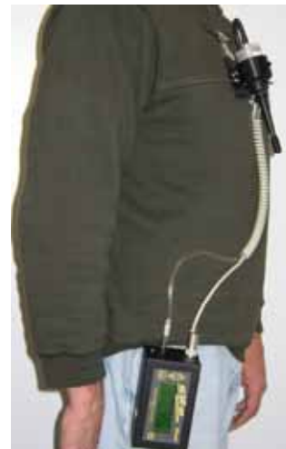
True Breathing Zone Measurements with Optical Infrared Sensor
